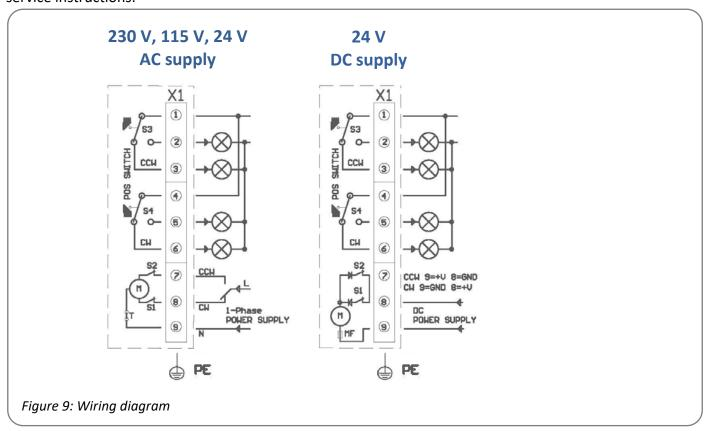
Two adjustable limit switches are installed to limit the stroke of the actuator, and cut-off the motor current in the relative direction.
