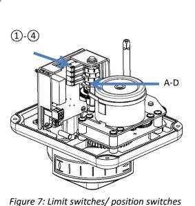
The limit switches are pre-adjusted in the factory.
