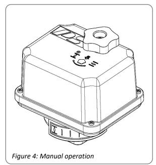
Do not exceed the adjusted electrical stroke limits by using the hand wheel.
