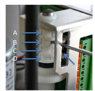
Figure 8: Setting the switching cams for the limit switches
