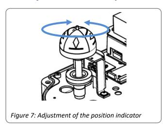
The position indicator is a two-coloured half ball turning under a transparent dome with blackened quarter segments.
