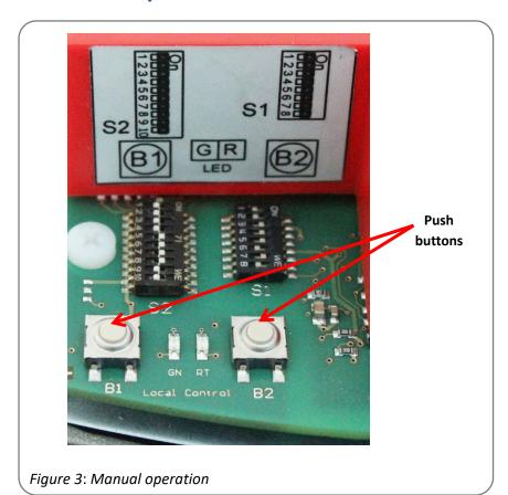
For commissioning the actuator during adjustment work (valve mounting and end position adjustment), an electrical manual override by means of a push-button is available (see 12.7 Manual operation).
