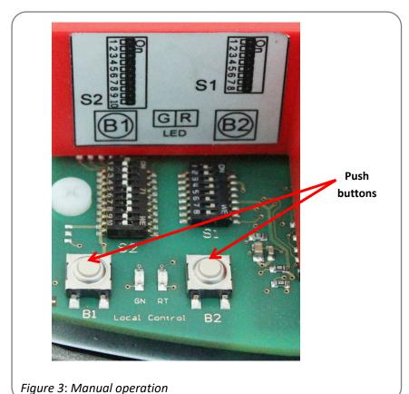
For commissioning the actuator during adjustment work (valve mounting and end position adjustment), an electrical manual override by means of a push-button is available (see 12.6 Manual operation).
