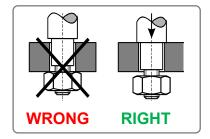
Before the pillar nuts are tightened, make sure that the pillars are sitting on the valve mounting bracket. If necessary, correct the position of the actuator by using manual operation. If these instructions are not observed, personal injury or damage to the actuator and/or valve may result.
