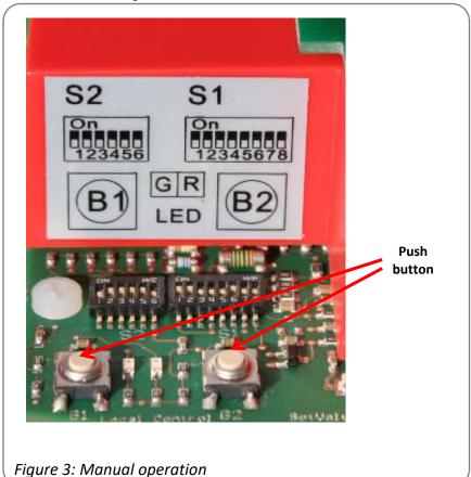
Two push buttons are installed to drive the actuator in case of installation work such as mounting onto a valve, or setting the limit switches positions (see 10.6).
