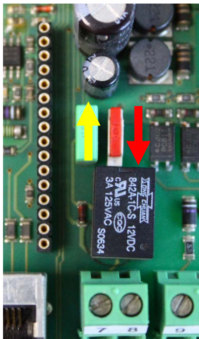
Figure 5: Slide switch for selecting the interface
