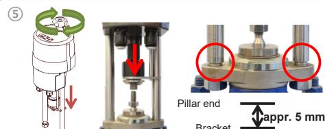
Move the coupling down until it hits the valve stem.
