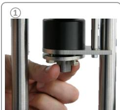
Make sure that the coupling nut can be turned by hand
