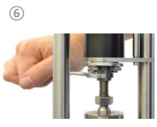
Screw the coupling nut onto the valve stem until the pillar edges rest on the bracket
